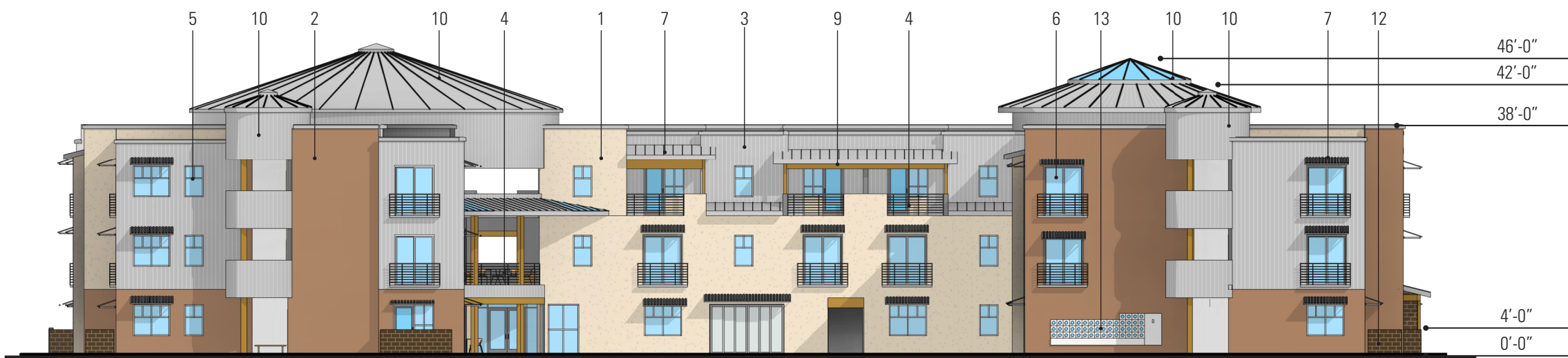
East Elevation - Courtyard 1/32" = 1'-0"
